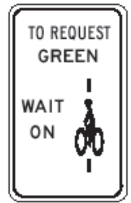
Fig. 7-29. Signage can help instruct bicyclists on how to use the detector loop.
