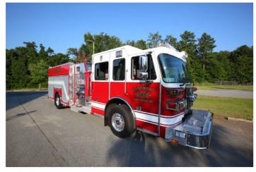
Engine 1 is a 2014 Sutphen Custom Cab Pumper/Tanker. It includes a 1500 gallon per minute Hale pump with a 1000 gallon booster tank.
