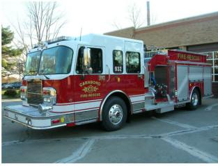
Engine 2 is a 2006 Elite Pumper/Tanker. It includes a 1500 gallon per minute Hale pump with a 1000 gallon booster tank.
