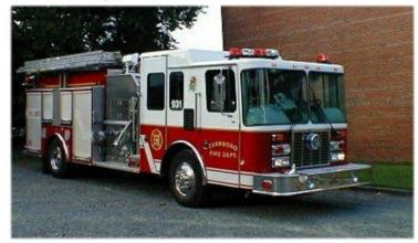
Engine 10 is a 1999 Ferrara Pumper/Tanker. It includes a 1500 gall per minute Hale pump with a 1000 gallon booster tank.
