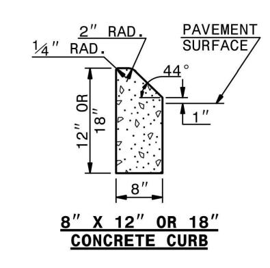
**CONCRETE MEDIAN AND CURB SECTION**
