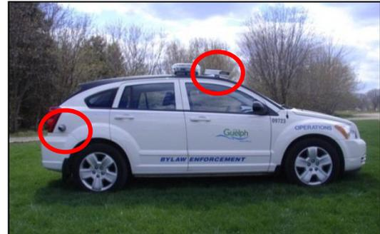
Parking enforcement vehicle with cameras highlighted
