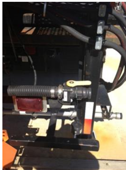
Picture # 2 Fill Valve # 2
