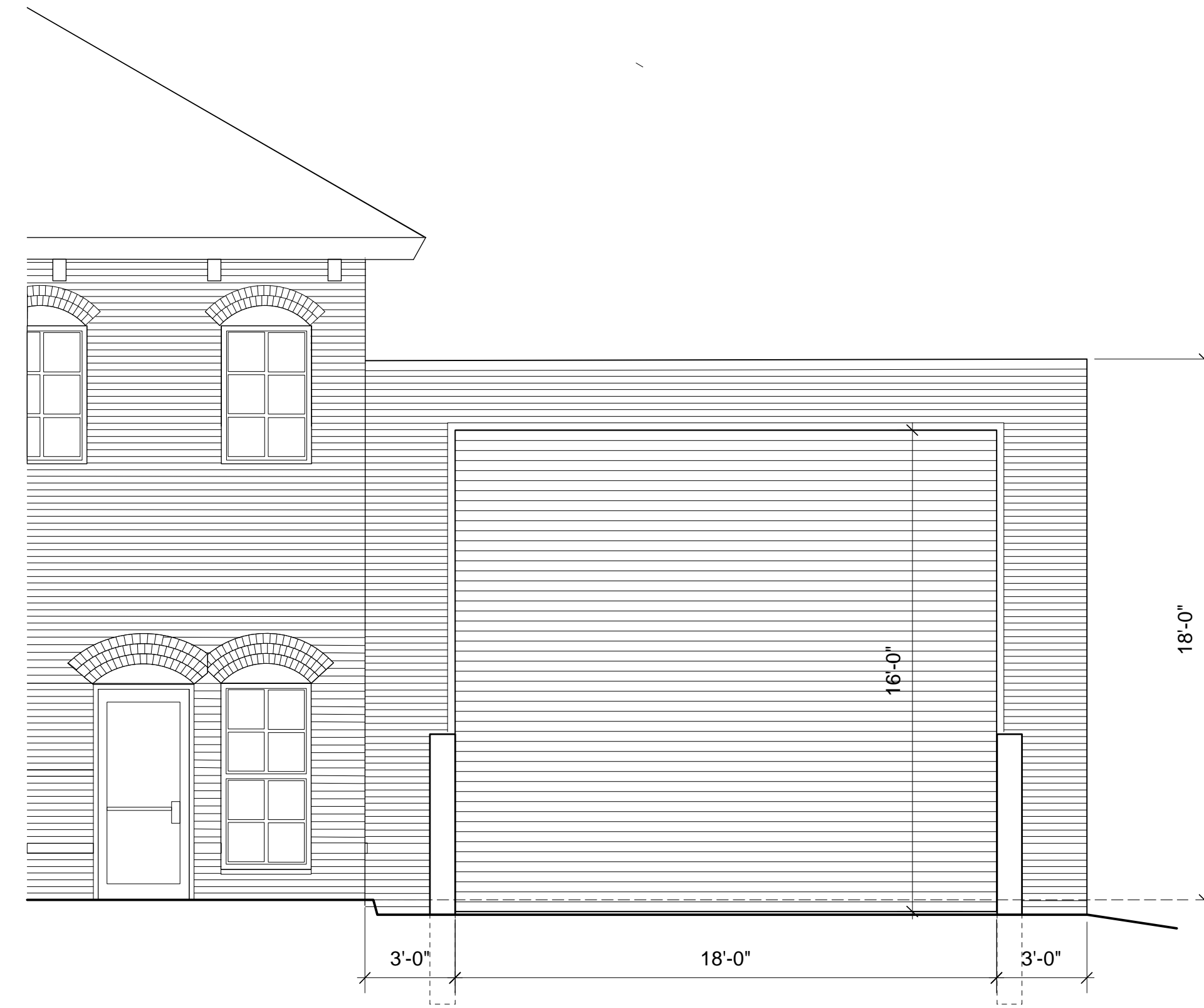
2 Dumpster Overhead Door Elevation Option 1 A-7.1 Scale: 1/4" = 1'-0"
