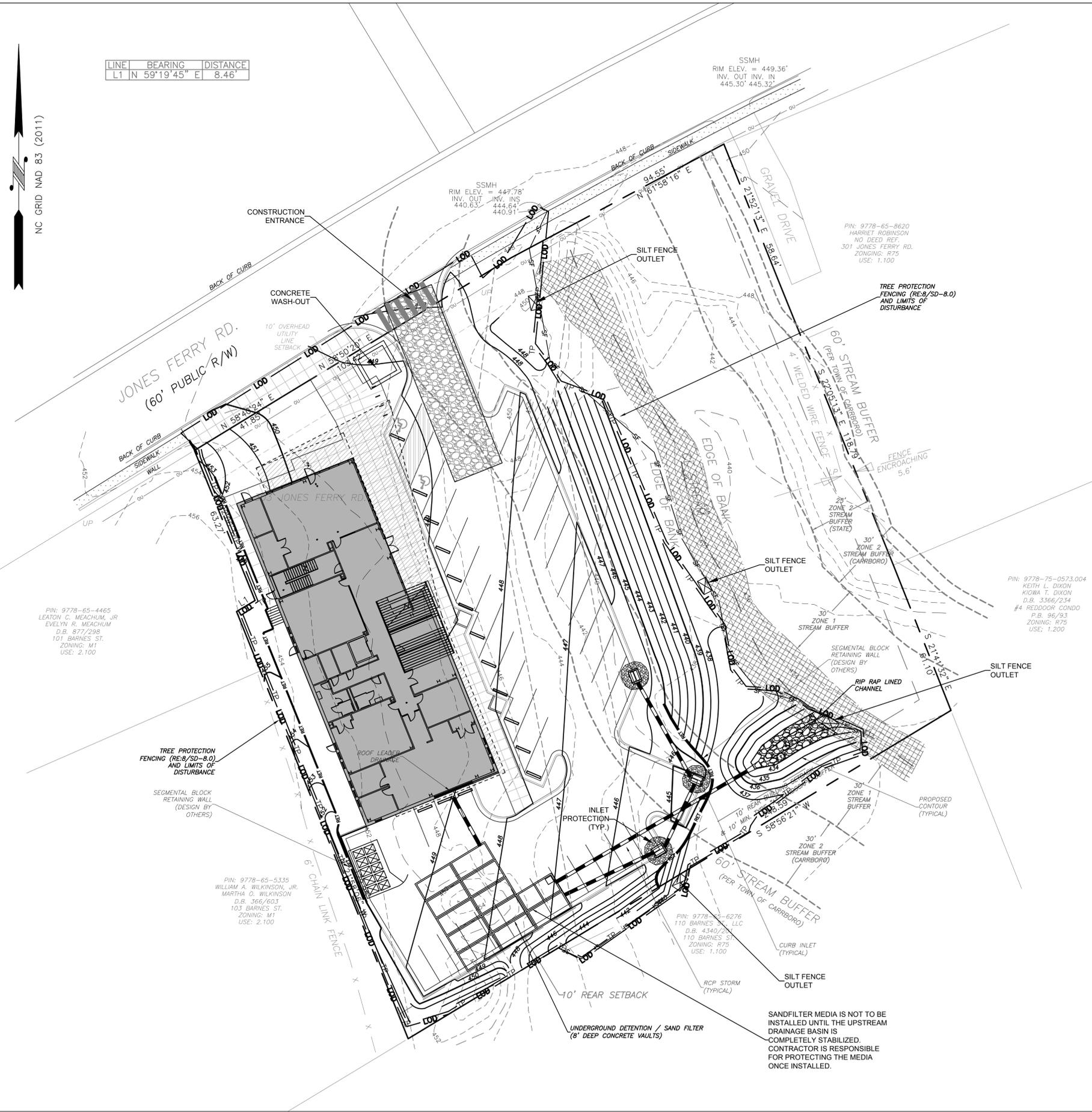
1. INSTALL SILT FENCE PRIOR TO WORK IN ANY AREA TO PREVENT SILT FROM LEAVING SITE.
