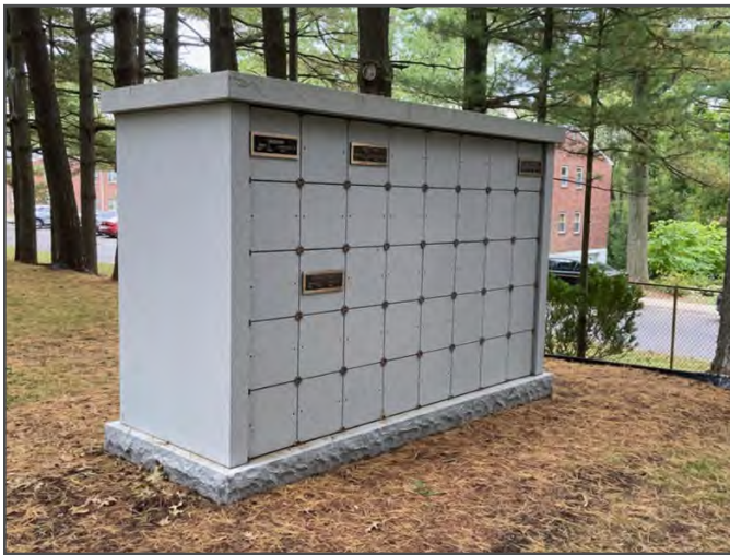
Figure 38 An 80-niche columbarium, faced in granite, with bronze markers on niches. The granite niche covers are pre-drilled to accept bronze plaques. (CVDA)
