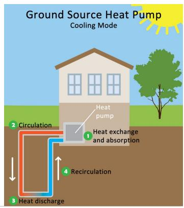
A Geothermal heating and cooling system (Source: EPA).
